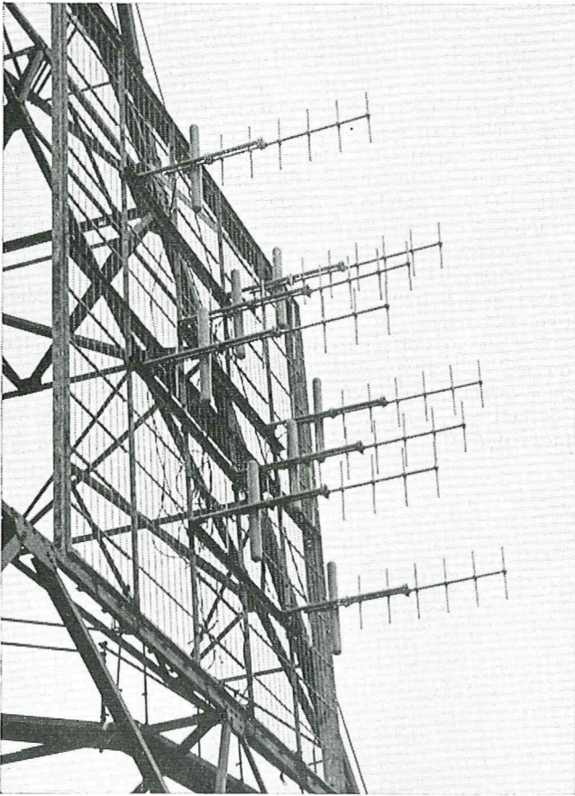
The photograph shows the aerial temporarily mounted for test purposes FIG. 4—One of the Channel 11 aerial arrays
